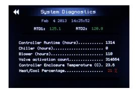
Real-time view of diagnostics helps maintain proper operation of equipment.
